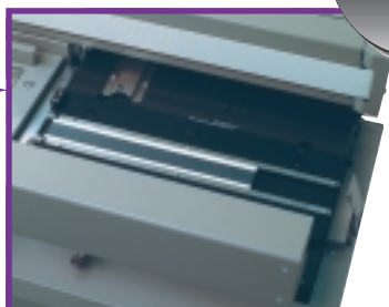
Placing a tape on the nipping station.
