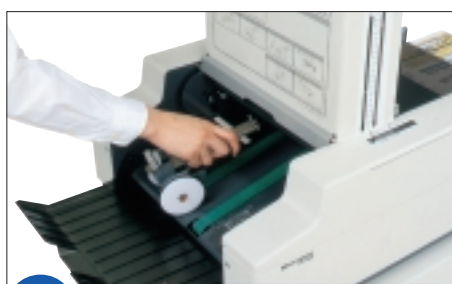
1 Remove the delivery roller.
